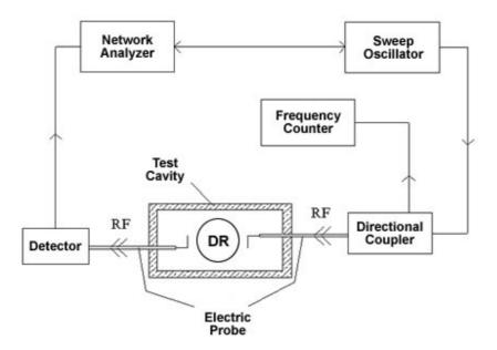
Figure 1. Experimental setup for measuring of the microwave parameters<sup>10,11</sup>.
