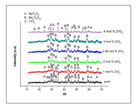
Figure 2. X-rays diffraction patterns for the ceramics synthesized and sintered at 1360°C.
