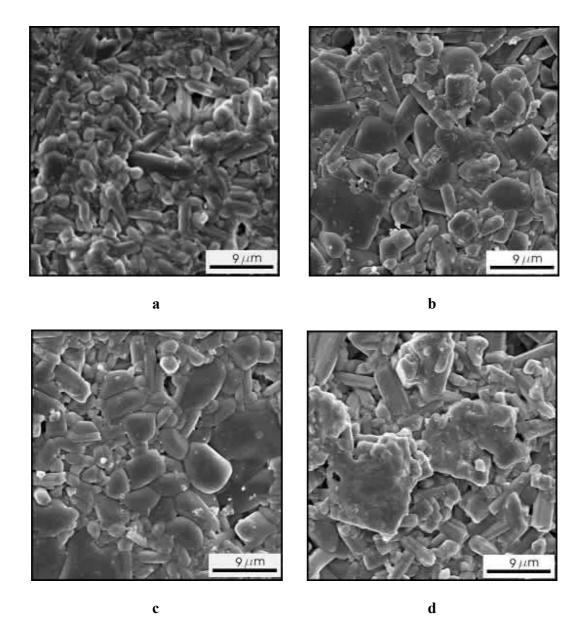
Figure 3. SEM images of fracture surface microstructure for the investigated ceramics: (a) B2T9 pure, (b) 2 mol % ZrO<sub>2</sub>, (c) 2.46 mol % ZrO<sub>2</sub>, and (d) 3 mol % ZrO<sub>2</sub>.
