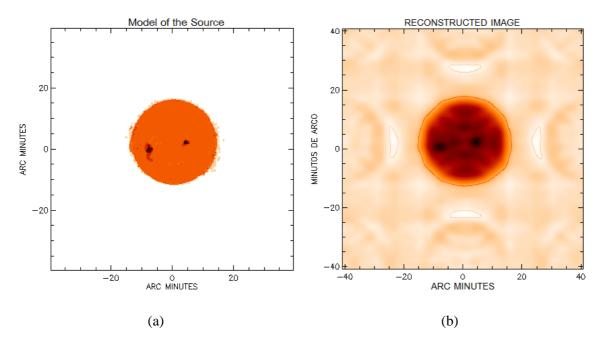
Fig. 5 - a) Image of Solar disc obtained from Nobeyama Radio Heliograph at 17 GHz that was used as a model of the Sun; (b) dirty image obtained with BDA configuration presented in Fig. 1.
