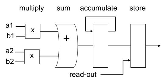
Fig. 2 – Design of a correlator cell. The inputs are the cosine and sine signals from a pair of antennas.
