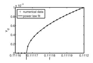
FIG. 11. The variation of the velocity with respect to the external force for a continuous transition ( $\delta_m$ =-0.50,  $V_0$ =0.207) for the  $c(2\times2)$  and the corresponding power law fit. The vertical arrow marks the value of the critical depinning force. The triangles represent the numerical data, while the continuous line the power law fit with  $\zeta$ =0.50  $\pm$  0.03.
