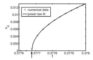
FIG. 7. Dependence of the velocity on the external force for a continuous transition for the  $(1 \times 1)$  phase  $(\delta_m = 0.125, V_0 = 0.0900)$ . The vertical arrow marks the critical force  $f_c$ . The triangles represent the numerical data, while the continuous line is a power-law fit with  $\zeta = 0.50 \pm 0.03$ .
