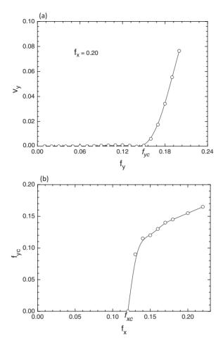
FIG. 14. (a)  $v_y$  as a function of an additional force  $f_y$  in the transverse direction, with  $f_x$  fixed. (b) Critical transverse force  $f_{cy}$  as a function of the longitudinal force  $f_x$ . Results for  $V_0$ =0.275,  $\delta_m$ =-0.5.
