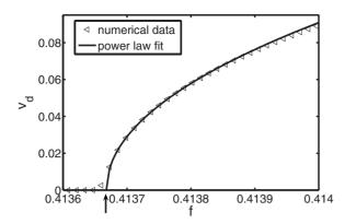
FIG. 3. Continuous depinning transition for relatively high pinning strength ( $\delta_m$ =0.3125 and  $V_0$ =0.250). The arrow marks the value of the critical depinning force. The triangles represent the numerical data while the continuous line is a fit to  $(f-f_c)^{\zeta}$ . The best fit is obtained for the exponent  $\zeta$ =0.50 ± 0.03.
