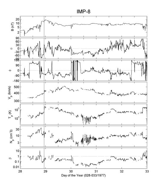
FIGURE 4.12 - Interplanetary shock observed by IMP-8 on DOY 28/1977, at 22:40 UT, identified by the vertical line. This is the same shock previously observed by H2 and later on by H1. The plots are given in the same sequence as the one in Figure 4.10. IMP-8 was in the solar wind near Earth during the period of observation of this shock.
