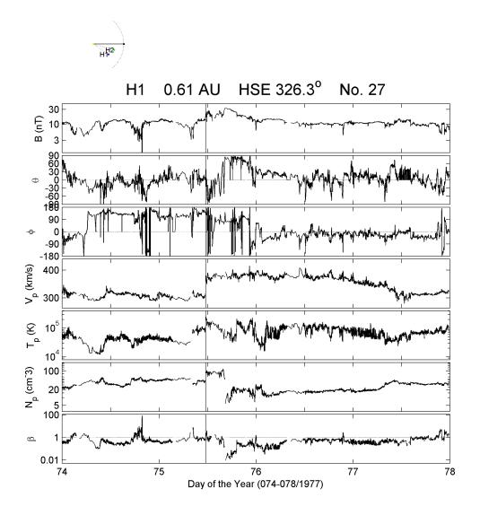
FIGURE 4.13 - A shock wave was detected by H1 on DOY 75 of 1977, at 11:33 UT, as identified by the vertical line. Plots are organized similarly as in Figure 4.10.
