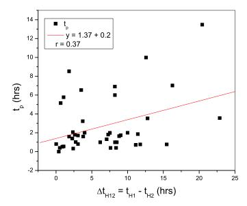
FIGURE 4.5 - Correlation between the difference on the shock speeds of H1 and H2 and the predicted time for the shock arrival. Note that  $\Delta t_{H12}$  comes from the measurements of H1 and H2, while  $t_p$  is predicted based on  $V_S = constant$ .
