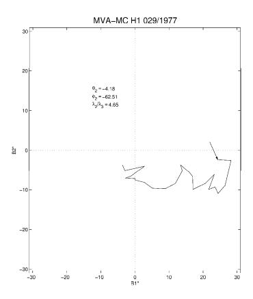
FIGURE 5.8 - Plane of Maximum Variance for the MC on DOY 029-030/1977 as observed by H1. The angles for the direction of the cloud's axis are represented by  $\theta_2$  and  $\phi_2$  in the figure. In addition, the error criteria  $(\lambda_2/\lambda_3 > 2)$  is satisfied. The arrow indicates the initial points and gives the direction of the rotation of the magnetic field.
