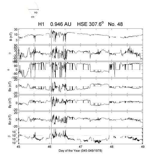
FIGURE 5.39 - H1 observation of a MC from DOY 046/1978, at 12:46 UT, to 047/1978, at 21:50 UT. The plots give, from top to bottom, the profiles of the magnetic field strength, inclination and azimuthal angles, the components  $B_x$ ,  $B_y$  and  $B_z$ , and the plasma beta, respectively. The vertical continuous line identifies the shock wave, driven by the MC whose boundaries are represented by the dotted lines.
