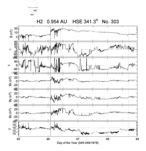
FIGURE 5.42 - H2 magnetic field data for the period from 044 to 048/1977. The plots give, from top to bottom, the profiles of the magnetic field strength, inclination and azimuthal angles, the components  $B_x$ ,  $B_y$  and  $B_z$ , and the plasma beta, respectively. The vertical continuous line identifies the shock wave, driven by the MC whose boundaries are represented by the dotted lines.
