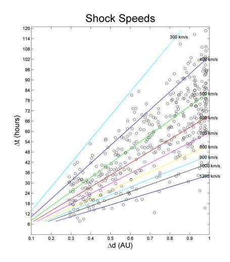
FIGURE 4.4 - Estimate of the arrival time of the shock waves as a function of the radial distance from the Sun according to Helios observation. The circles ( $\circ$ ) that fill the plot are the result of the shock speed measurements of Helios probes. Each circle corresponds to a shock speed calculated when the shock was detected at a determined radial distance (AU), based on the remaining distance.
