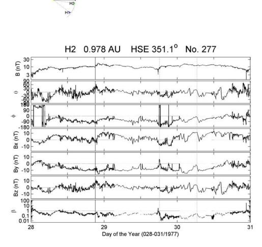
FIGURE 5.6 - H2 magnetic field data for the period on DOY 29/1977. The plots give, from top to bottom, the magnetic field strength, inclination and azimuthal angles, and components  $B_x$ ,  $B_y$  and  $B_z$ , followed by the plasma beta, respectively. The vertical continuous line identifies the shock wave, driven by the MC whose boundaries are represented by the dotted lines.
