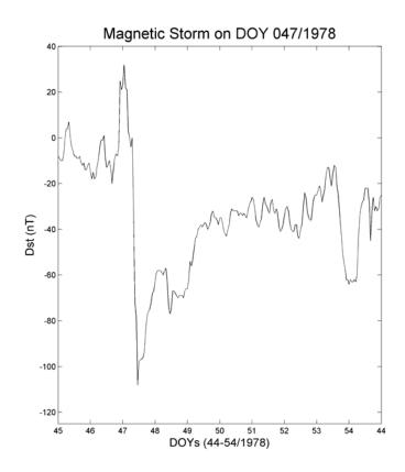
FIGURE 5.44 - Intense magnetic storm ( $Dst_p = -108 \ nT$ ) registered on DOY 047/1978 at the terrestrial magnetosphere.
