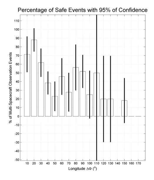
FIGURE B.3 - Percentage of shocks observed by multi-spacecrafts and the error margin estimated for the percentage of shock waves observed in each angular separation  $\Delta\Phi$  based on the test for proportions.
