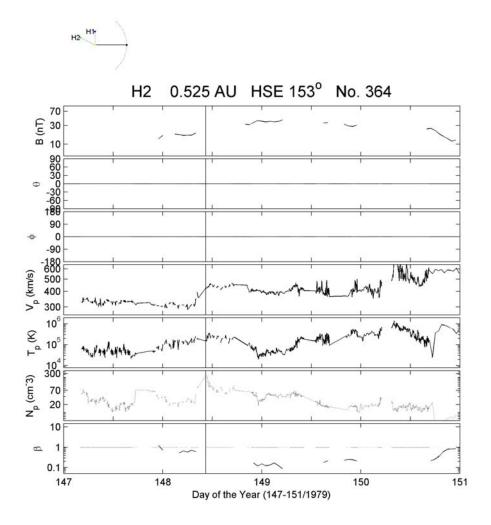
FIGURE 4.15 - H2 observation of a shock wave on DOY 148/1979, at 10:28 UT, as identified by the vertical line. The plots are given in the same sequence as in Figure 4.10. Even with gaps on the data, one can identify some of the features for a possible MC.
