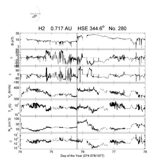
FIGURE 4.14 - H2 observation of a shock wave on DOY 75/1977, at 19:47 UT. The plots are given in the same sequence as in Figure 4.10. The shock is identified by the vertical line. It is driven by an ICME/MC, like the low plasma beta and density show.
