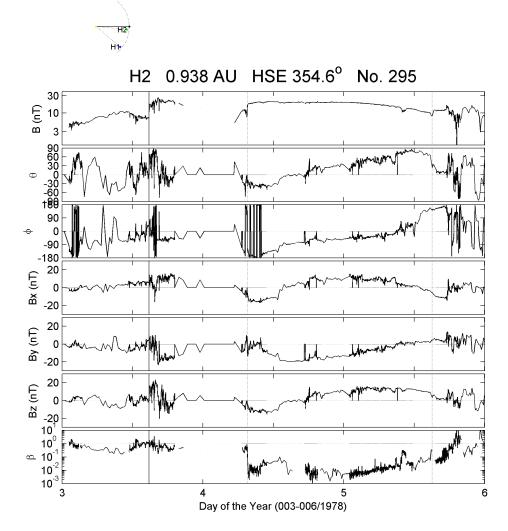
FIGURE 5.32 - H2 magnetic field data for the period from 003-006/1978. The plots give, from top to bottom, the profiles of the magnetic field strength, inclination and azimuthal angles, the components  $B_x$ ,  $B_y$  and  $B_z$ , and the plasma beta, respectively. The vertical continuous line identifies the shock wave, driven by the MC whose boundaries are represented by the dotted lines.
