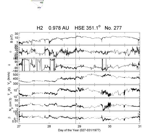
FIGURE 4.11 - H2 observation of a shock on DOY 28/1977, at 21:07 UT. The plots are organized similarly to Figure 4.10. This is the same shock as seen in H1, however, the signatures for a MC are not visible as they are in H1.
