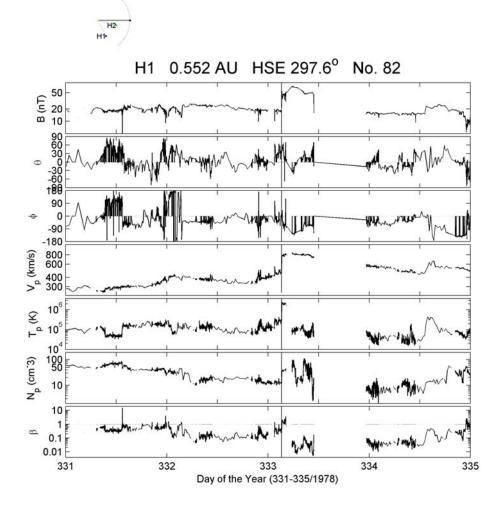
FIGURE 4.25 - H1 observation of a shock wave on DOY 333/1978, at 03:17 UT, as identified by the vertical line. The plots are given in the same sequence as in Figure 4.10.
