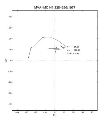
FIGURE 5.25 - Maximum Variance plane for H1 observation of a MC on DOY 335/1977. Through intermediate variance, the angles  $\theta_2$  and  $\phi_2$  that represent the direction of the cloud's axis are obtained. The arrow indicates the initial points and gives the direction of the rotation of the magnetic field.
