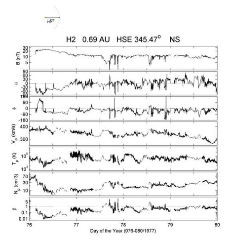
FIGURE 4.21 - H2 solar wind and magnetic field profiles for the period from DOY 76 to 80/1977. The plots are given in the same sequence as in Figure 4.10. No shock (NS) signatures are registered for the considered period.
