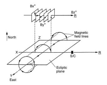
FIGURE C.1 - Representative sketch of a magnetic flux tube (approximation for a MC). traveling in the IP medium. Note that the original coordinate system is changed due to the application of the MVA technique, resulting in the components of maximum  $(B_x^*)$ , intermediate  $(B_y^*)$ , and minimum  $(B_z^*)$  variance of the magnetic field.
