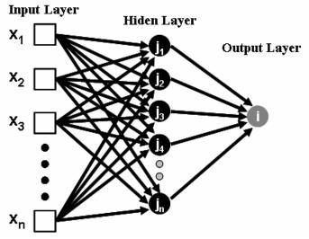
Figure 2 - Architecture of multi-layer perceptron.
