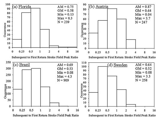
**Figure 3.** Histogram of the ratio of the subsequent-to-first-return-stroke electric field peak for multiple-stroke negative cloud-to-ground lightning flashes in (a) Florida, (b) Austria, (c) Brazil, and (d) Sweden.
