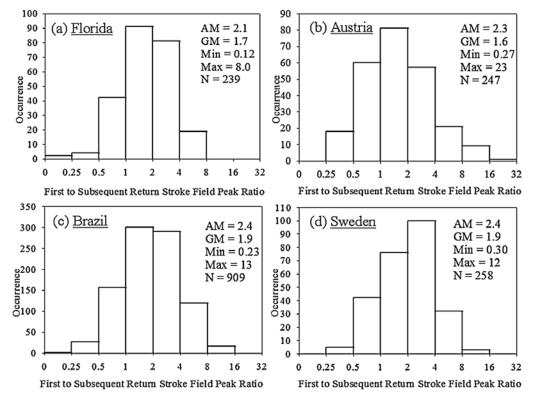
**Figure 2.** Histogram of the ratio of the first-to-subsequent-return-stroke electric field peak for multiple-stroke negative cloud-to-ground lightning flashes in (a) Florida, (b) Austria, (c) Brazil, and (d) Sweden.
