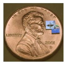
Figure 1.2 - Sensor nodes. Left side: "Spec" mote (by University of California- Berkeley). Rigth side: Golem Dust, one of the generations of sensors of the Smart Dust Project.
