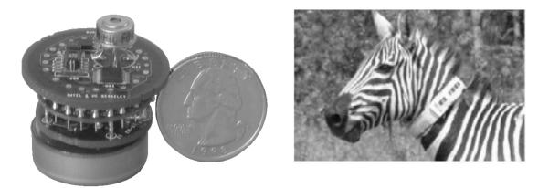
Figure 1.3 - Sensor nodes deployed by the projects *Great Duck Island* and *ZebraNet* Project (left and right side, respectively). Left side: MICA-2 (by Intel and University of California- Berkeley). Rigth side: Sensor necklace.
