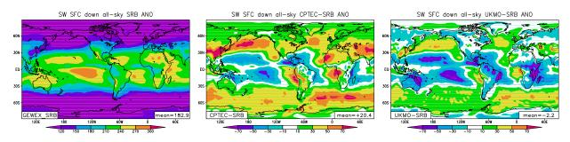
**FIGURE 3.** Annual mean of the all-sky incident short wave at surface (Wm<sup>-2</sup>). Left: generated by SRB project; middle: difference from SRB of current CPTEC AGCM; right: difference from SRB of CPTEC AGCM with UKMO code.
