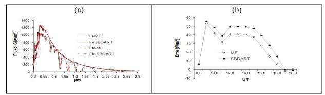
FIGURE 2. Quixerê, NorthEast Brazil, clear atmosphere. (a) Spectral fluxes calculated with the model (ME) and with SBDART (Fi: incident on top of atmosphere; Ftr: transmitted at ground level). Parameters: Rs= 0.15, aerosol load  $\tau(0.55) = 0.12$ ,  $\mu_0 = 0.62$  and  $w_{H20} = 2.0$  g.cm<sup>-2</sup>. (b) Daily cicles of deviation from measured global irradiance (UT: universal time).
