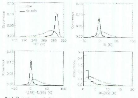
FIG. 2. Distributions from the four tests used in the screening routine for rain and nonrain pixels (based on the PR classification): PCT, scattering index,  $T_{V19} - T_{V85}$ , and std dev of  $T_{V85}$ . Thin (thick) line indicates rain (no-rain) pixels; bin size is 1 K.
