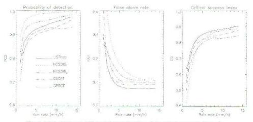
FIG. 8. POD, FAR, and CSI evolution as function of the PR observed surface rain.
