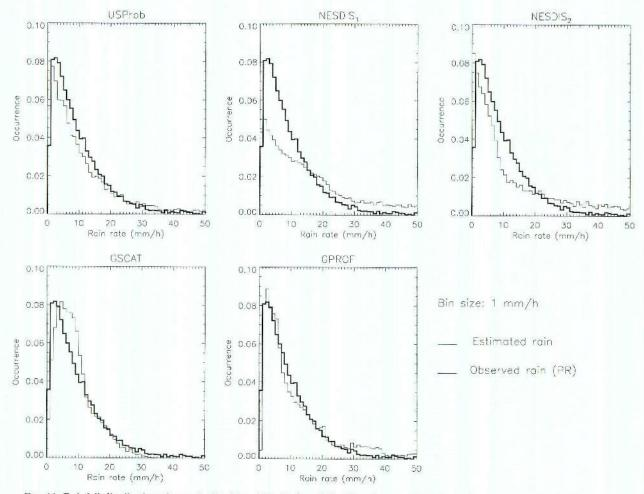
FIG. 11. Rainfall distributions for each algorithm (thin line) and the PR reference (thick line). From upper left to bottom right: USProb, NESDIS<sub>1</sub>, NESDIS<sub>2</sub>, GSCAT, and GPROF. Bin size is 1 mm h<sup>-1</sup>.
