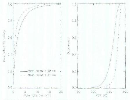
FIG. 1. (left) Rainfall rate and (right) 85-GHz PCT frequency distribution for rain systems that are larger than 69 km or smaller than 31 km in radius.
