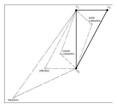
Figure 1. Nelder-Mead simplex method and the representation of new points in search space.
