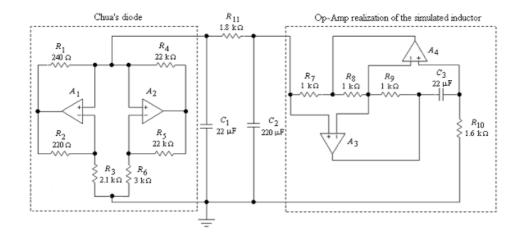
Figure 3. Implementation of Chua's oscillator.
