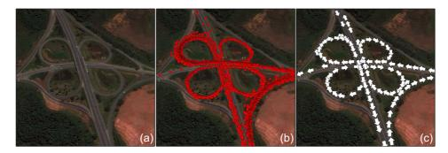
Figure 1. First test: (a) satellite image, (b) points after preprocessing, (c) road centerlines
