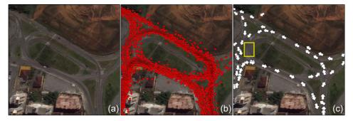
Figure 2. Second test: (a) satellite image; (b) points after preprocessing; (c) road centerlines with incorrectly mapped area highlighted
