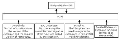
Figure 4. Requirements of the PGXS architecture
