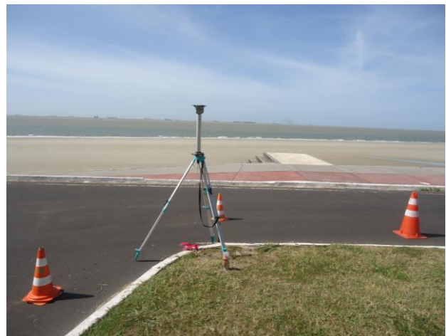
Figure 05 – Collection of control points during field survey.
