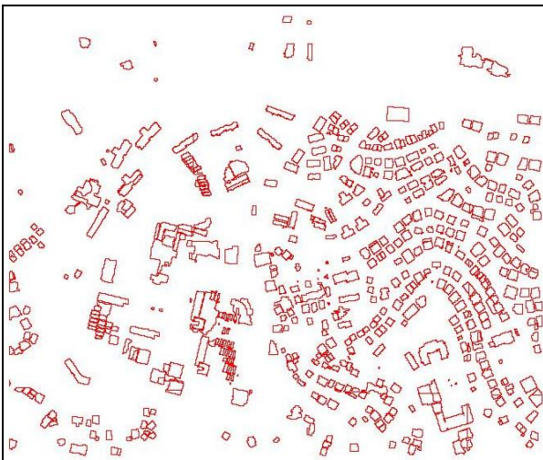
Figure 5a. Vector results of object-based classification of buildings from QuickBird image of 2004
