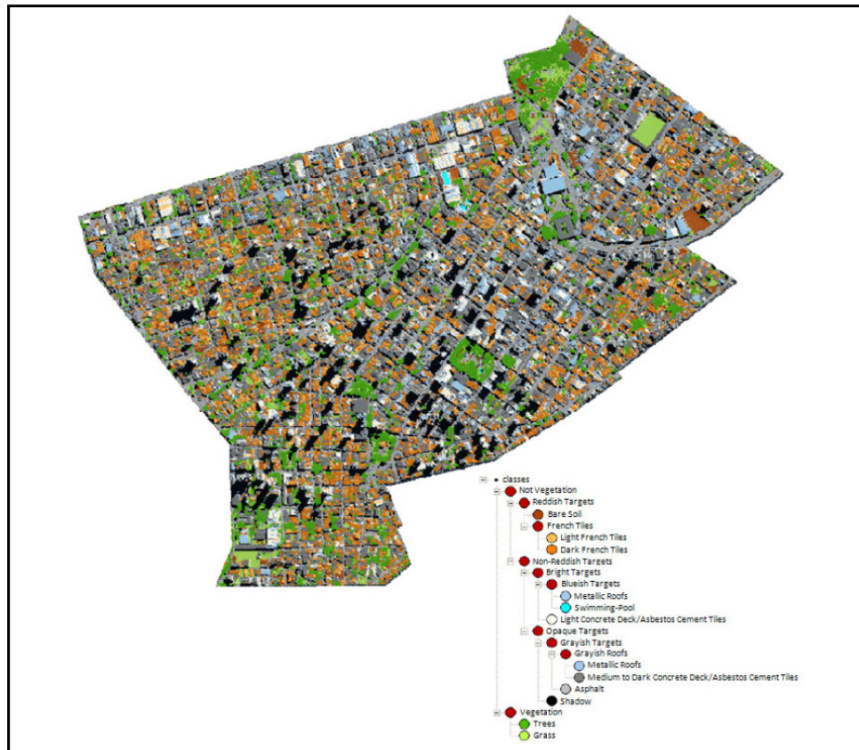
Figure 6. Object-based classification of urban land cover for the study area and its respective hierarchical semantic network derived from the generated decision tree
