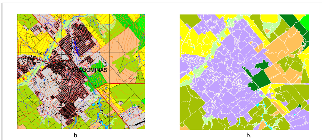
Figure 6. a. Inset of the thematic map (reference map) manually executed by photo-interpretors of OrbiSat (2007b) and containing the study area b. Final classification result for the study area produced by InterIMAGE (Color legend is found in Figure 3)
