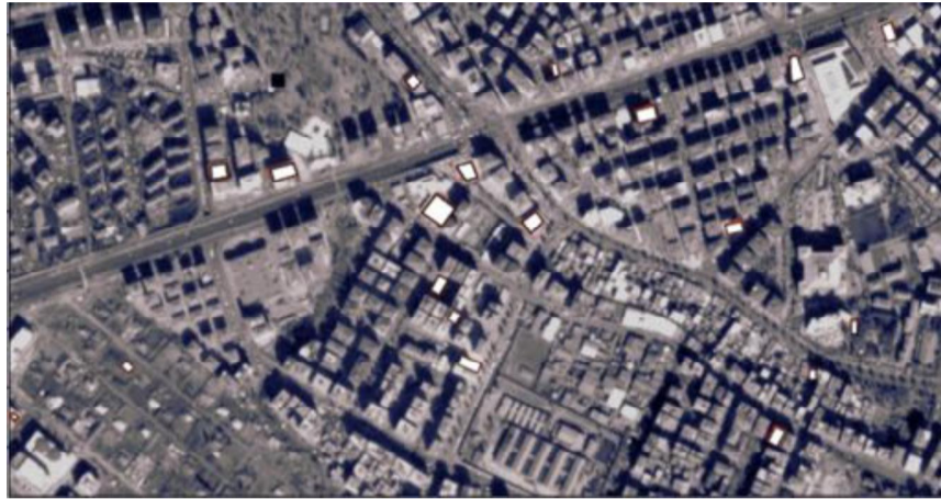
Figura 10. Shapefile Layer Buildings - Detected Changes. The polygons highlighted in the image represent the buildings that were identified as detected changes after the earthquake.
