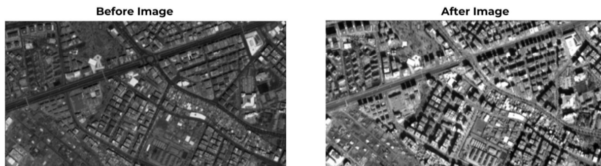
Figura 3. Images of the differences in brightness and contrast between bands 1 (left) and 4 (right) of the CBERS-4A satellite image from 2021.
