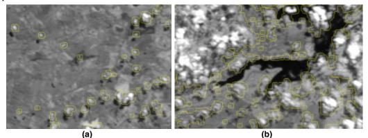
Figure 2. FMASK detected clouds and shadows where detected areas are enclosed by yellow color lines. In (a) shadows are not detected and in (b) some areas are detected as clouds although they are valid targets.
