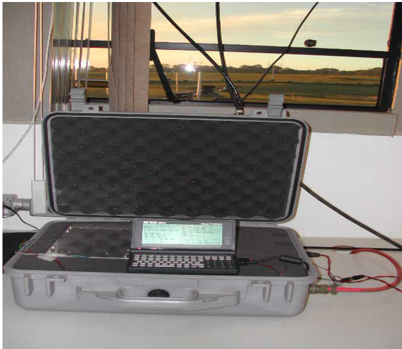
Figura 4: Magnetometro fluxgate instalado no OES/CRSPE/INPE - MCT
