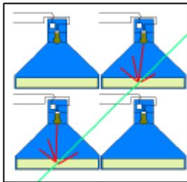
FIGURE 1 – An esquematic vision in vertical flat of the prototype muons detector showing the arrival direction of one muon in scintillation material and its detection by a photomultiplier.
