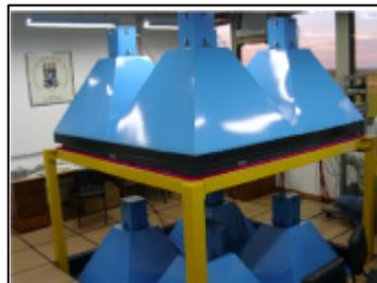
FIGURE 2 - A photograph of the prototype muons detector during May 2005 showing the eight detectors in the observation room.
