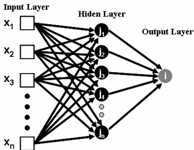
Figure 2 - Architecture of multi-layer perceptron.
