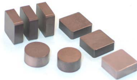
Fig. 4. Photograph of α-SiAlON cutting tools development in Brazilian laboratory.
