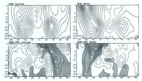
Fig. 4. Climatological vertical structure of zonal wind (m s<sup>-1</sup>) for the NEW model during (a) DJF and (b) JJA. Differences between the NEW and OPE models in (c) DJF and (d) JJA. Positive values are shaded in gray.
