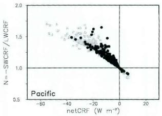
Fig. 11. Scatterplot of  $N \times$  netCRF from SRB satellite-derived observations (black) and the NEW model (gray) for DJF. Each point corresponds to a grid point over the tropical western Pacific region (10°N-5°S and 117.5°-170°E).
