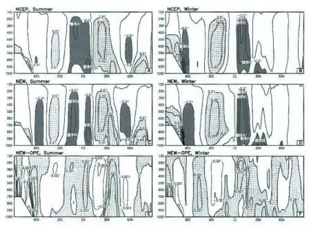
FIG. 5. Zonal mean vertical p velocity (Pa s<sup>-1</sup>) for (a), (b) NCEP-R and (c), (d) the NEW model, during (left) DJF and (right) JJA. (e), (f) The differences between the NEW and OPE models, where positive p-velocity differences are shaded in gray.
