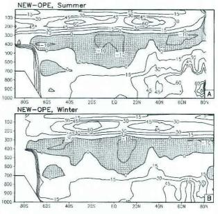
FIG. 2. Zonal mean shortwave heating rate difference (%) between the NEW and OPE models during (a) DJF and (b) JJA. Negative values are shaded in gray.
