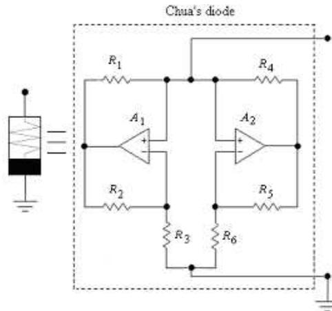
Figure 2. Representation of Chua's diode (Tôrres and Aguirre, 2000).
