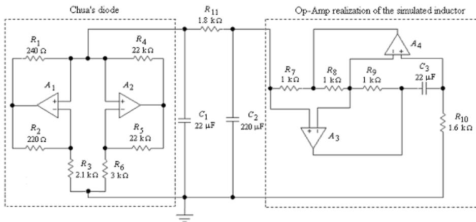
Figure 3. Implementation of Chua's oscillator.
