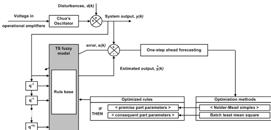
Figure 4. One-step ahead forecasting using T-S fuzzy model using NMO and batch mean least squares.
