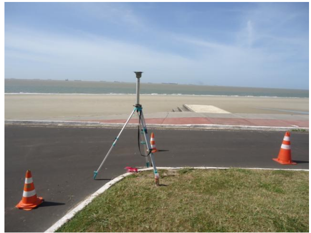
Figure 05 – Collection of control points during field survey.
