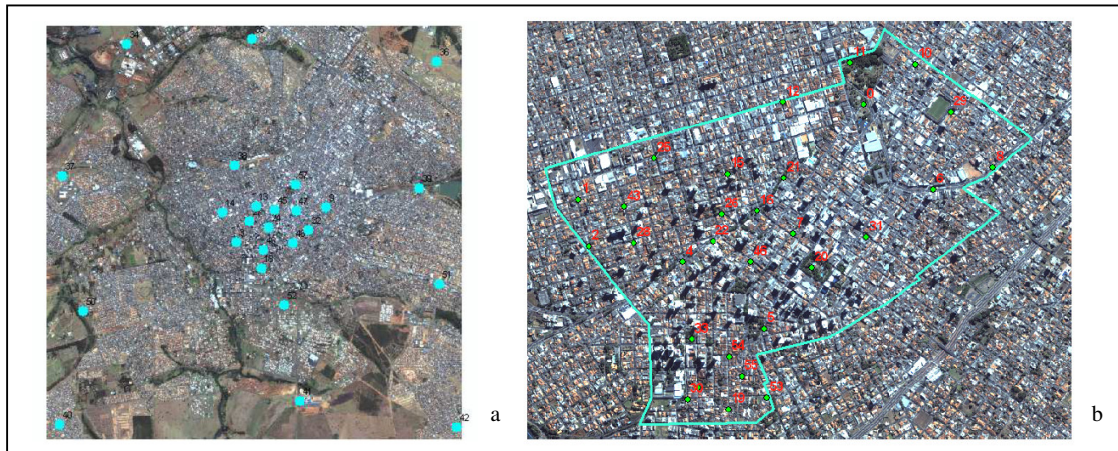
Figure 2. IKONOS II image orthorectification: a. The entire scene comprising the study area, with tie points (blue dots) used for orthorectifying the image, with their respective ID number in black b. Zoom in the scene, showing the study area boundaries (light blue line) and the validation points (green dots) with their respective ID number in red
