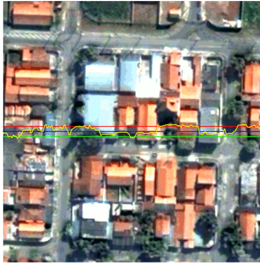
Figure 3. The adapted tile line (yellow) for the first example. Red and Green lines shows the buffer size (parameter t_2 ), and the Blue line shows the original tile line.
