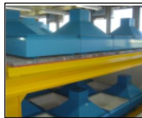
FIGURE 3 -A photograph of part from the extended multidirecional muons detector under construction during November 2005. It shows the upper layer, the lower layer and between them a 5 centimeter lead layer.
