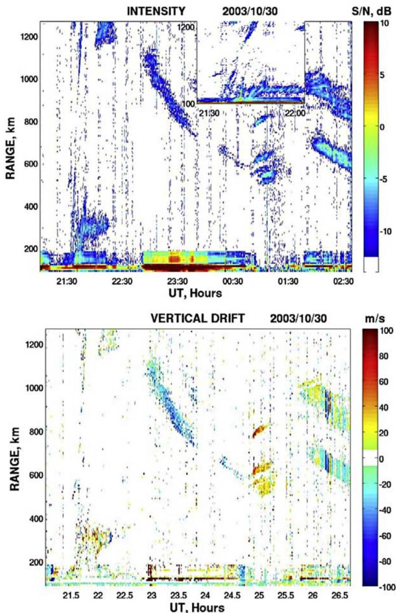
**Figure 3.** RTI (upper) and RTV (lower) maps from a 30 MHz coherent backscatter radar at São Luís on the night of 30 October. Note the rapid uplift of the 5-m irregularity echo patch near 21:30 UT (18:30 LT) (amplified in the inset). The vertical velocity of the uplift is calculated as  $\sim 1200$  m/s. The radar echo is weak on this night.
