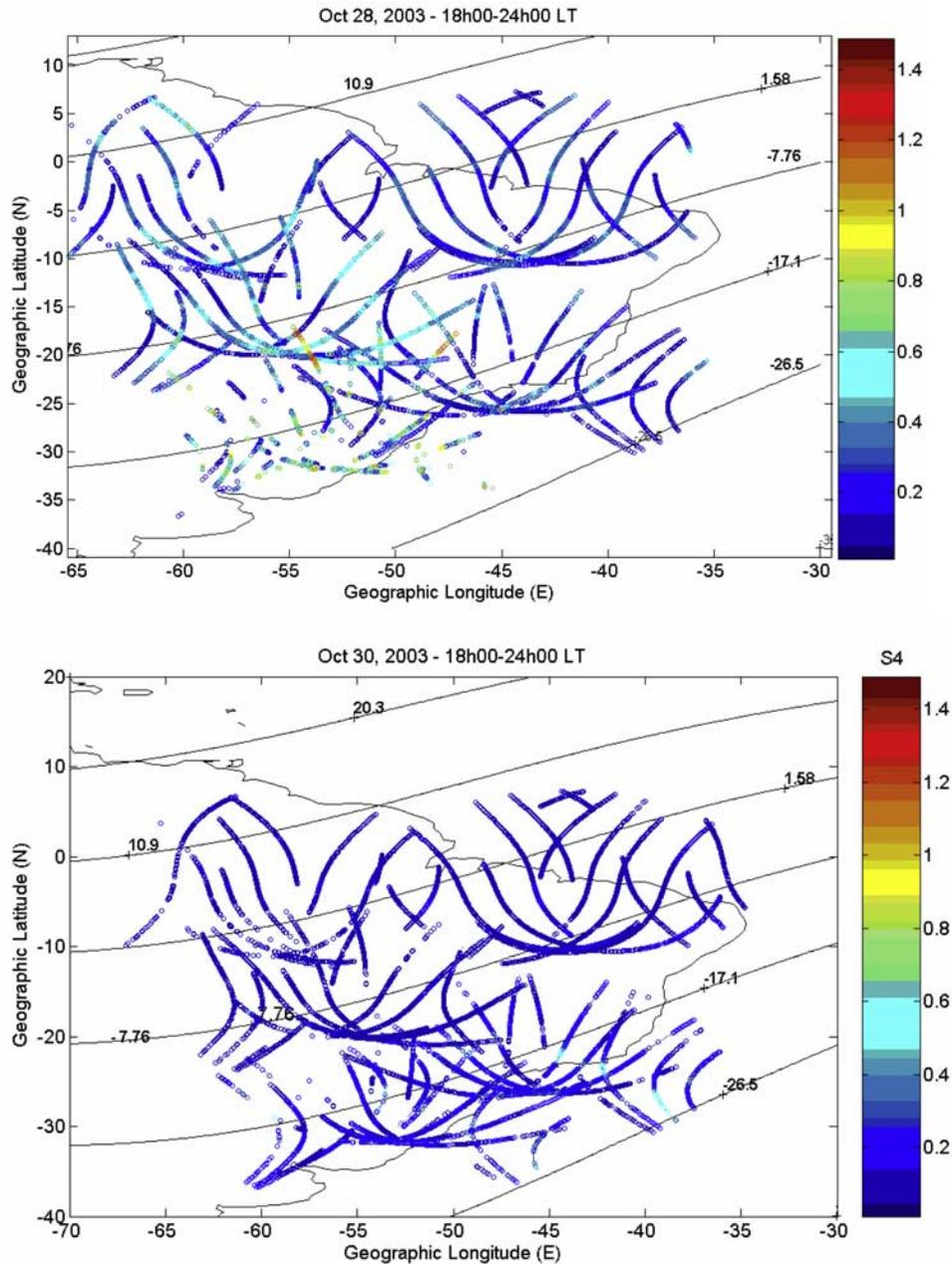
**Figure 4.** GPS Scintillation S4 index distribution in geographic latitude versus longitude on 28 October (reference day) and on 30 October. The S4 intensity is represented by the color code on the GPS orbital segments according to the color scale shown on the right.
