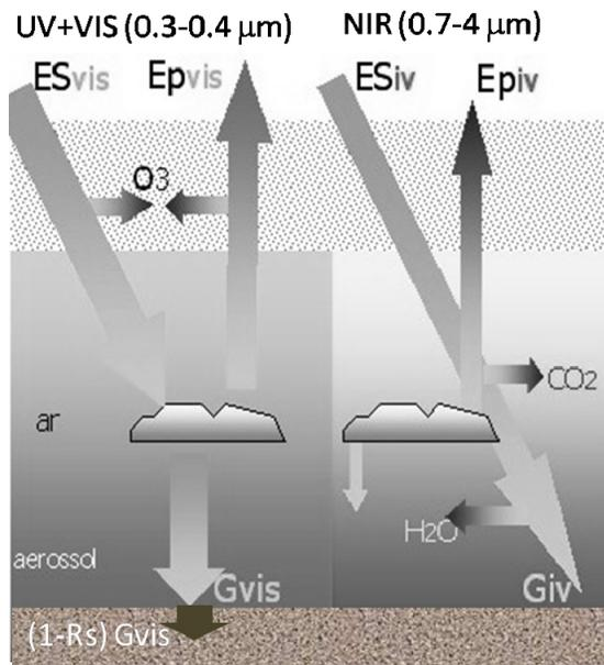
**FIGURE 1.** Schematic structure of GL/CPTEC model for solar radiation assessment by satellite
