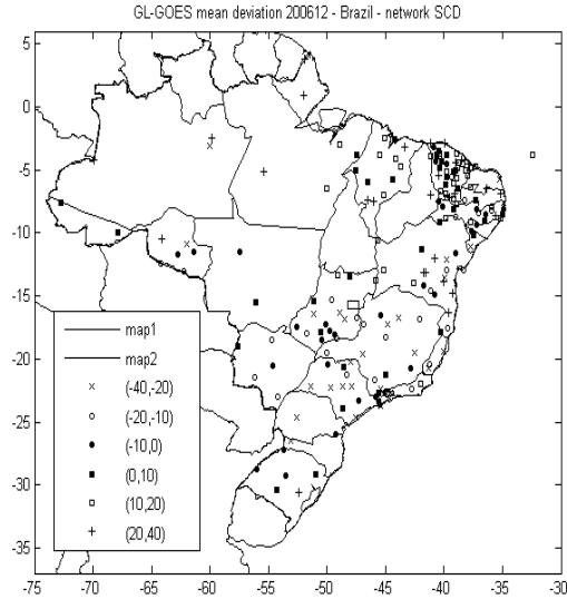
**FIGURE 2.** Validation of monthly GL results comparing with a pyranometric network. Symbols indicate difference of GL related to network value.
