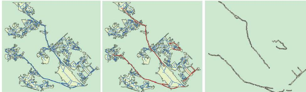
Fig. 7. Result of complex object. Left: Initial skeletons extracted with Method in[10]. Middle: Result of skeleton decomposition, where road parts are marked with red lines. Right: road regions reconstructed with the average width of skeleton segments.
