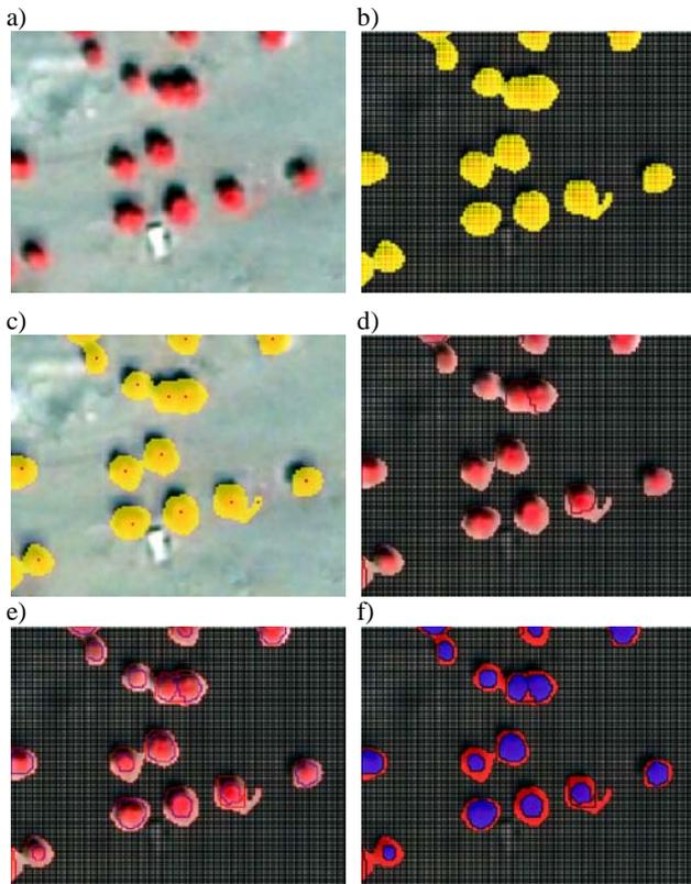
Figure 3: Object based image analysis procedure for single crown identification and delineation, a) QB scene (NIR1, red, green), b) chessboard segmentation, c) find local extrema, d) multiresolution segmentation region grow, e) contrast split segmentation, f) classification result
