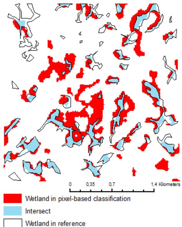
Figure 4. Overlapping Maximum Likelihood Classification (MLC) polygons (in red), reference base (black line) and intersect (in blue).
