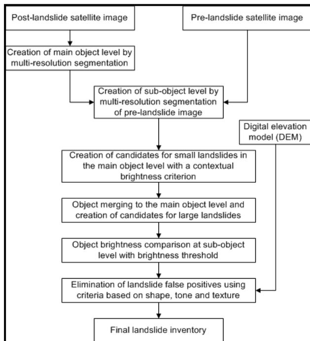
Figure 2. Methodology flowchart for detection of landslides from panchromatic images.
