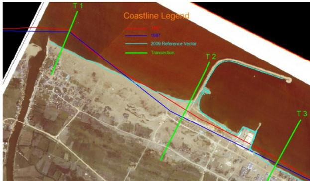
Figure 5. Comparison of object-based vector results, manual on-screen digitising vector results and reference vector; **blue**: object-based results, **red**: manuel on-screen digitizing, **cyan**: reference vector, **green**: transections
