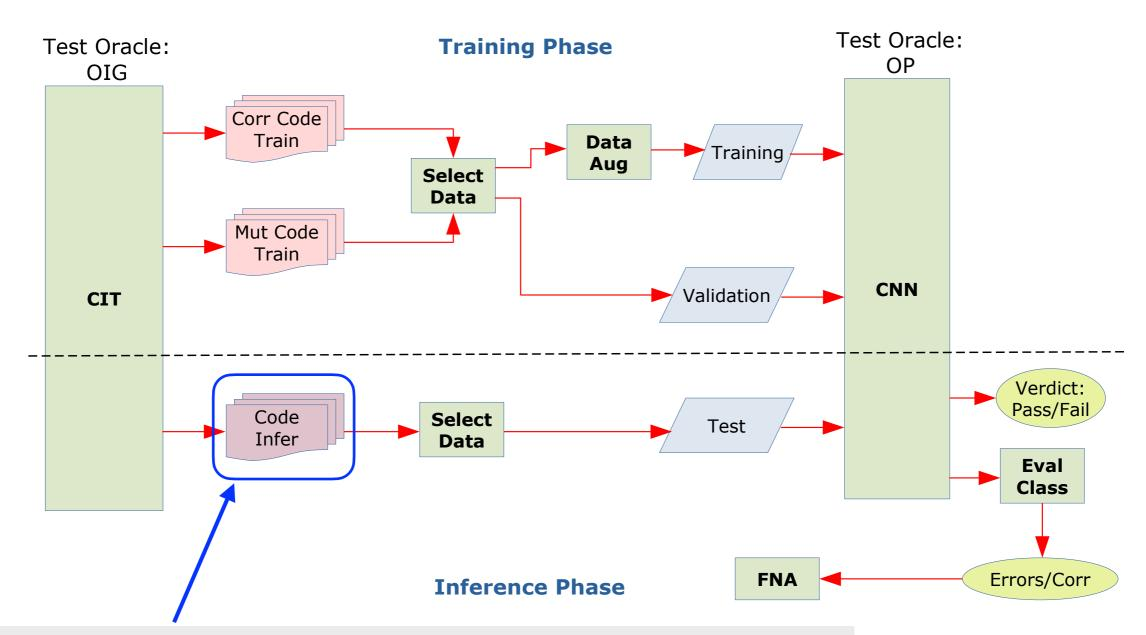
Test set is created based on the outputs of programs completely different from the ones used to create the training and validation sets.
