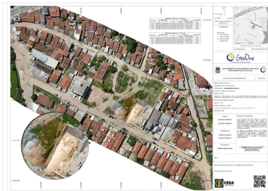
Figure 8. Survey plan with drone's orthoimage ( click on the picture to see it in full size ).
