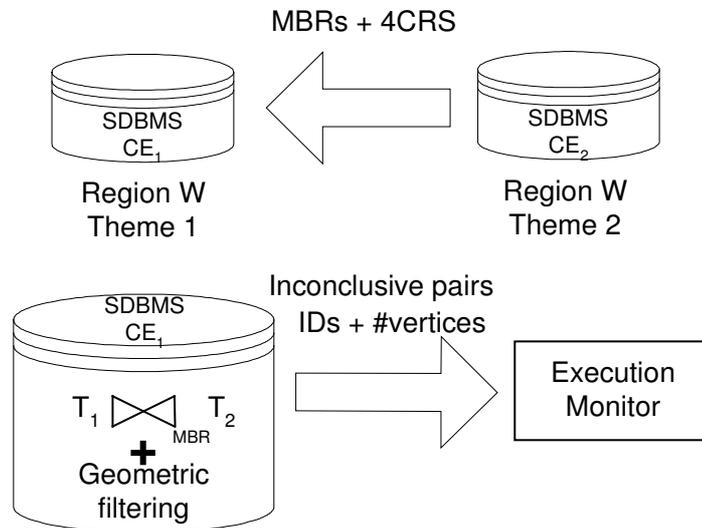
**Figure 4. Sub-queries' running sequence in CEs with SDBMS**
