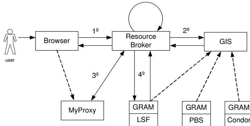
**Figure 1. Resource Broker acting as a middle tier in a grid - adapted from (Afgan 2004)**
