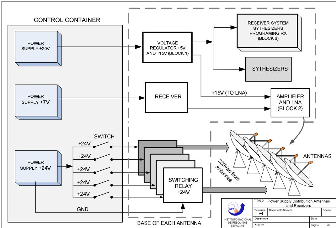
Figure 1 - BDA's receiving section simplified block diagram
