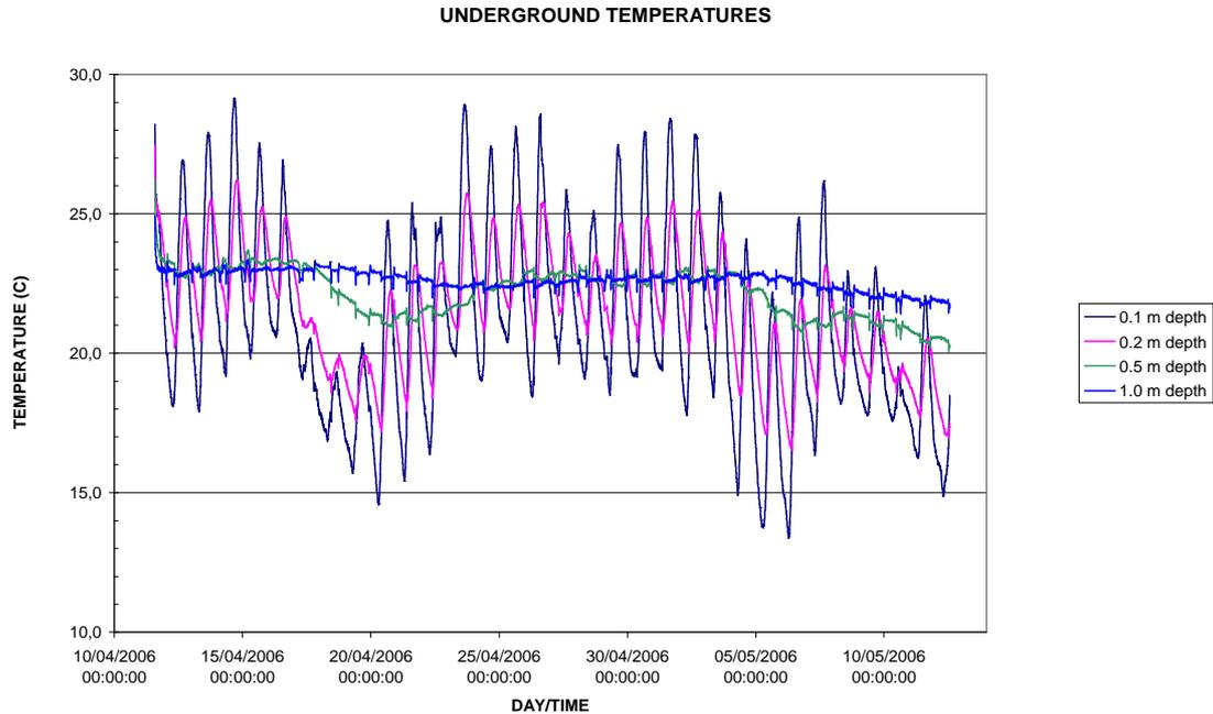
Fig. 3 - Actual temperature monitoring at different depths.
