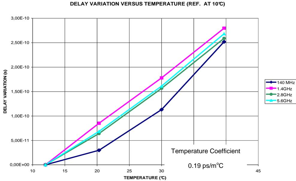
Fig. 2 - Phase delay measurements for cable datalink RGC213.
