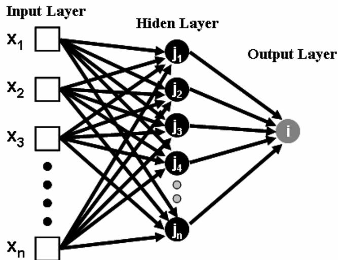
Figure 2 - Architecture of multi-layer perceptron.
