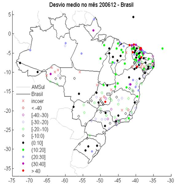
**FIGURE 2.** Validation of monthly GL results comparing with a pyranometric network. Colored circles indicate difference of GL related to network value.
